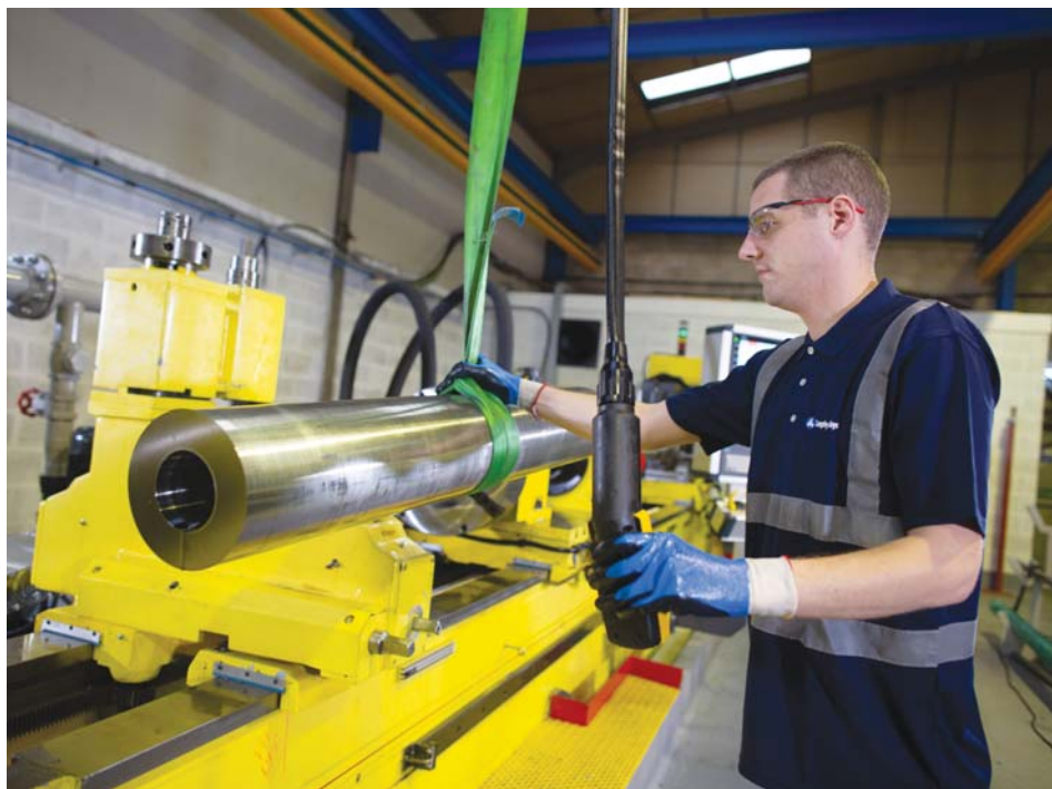
Additional in-house services include deep hole boring, machining and CNC-controlled bands saws, capable of accurate stock cutting up to a section size of 500mm (20").
