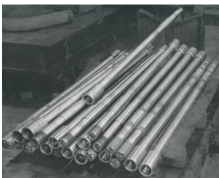
The development of North Sea oil in the UK led to a surge in the requirements for newer alloys with greater levels of performance. Here are components for line shaft pumps specified in Ferralium as an alternative to Alloy K-500.
